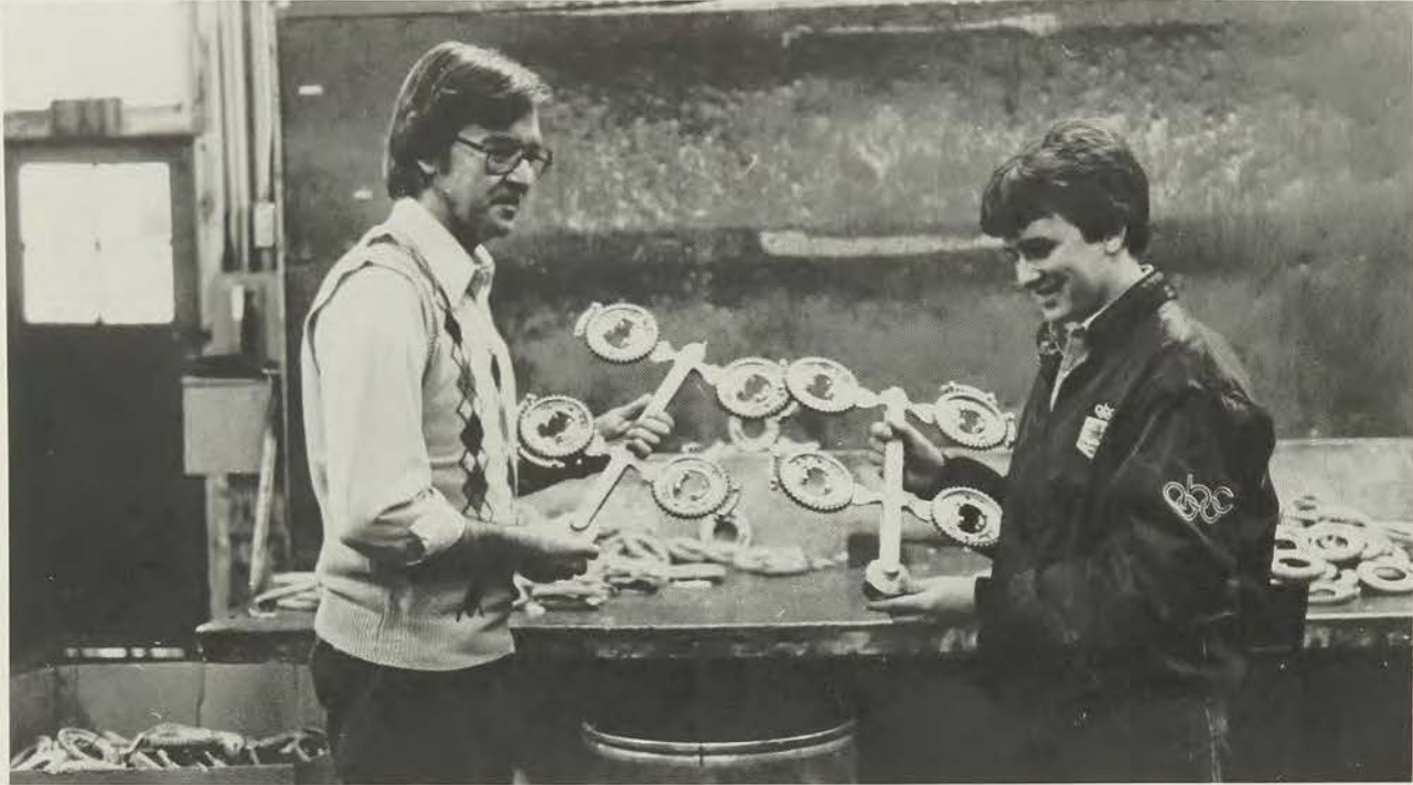
An employee shows sophomore Tony Key the timing gear that Alpha Industries produce for V6 Buick engines.
